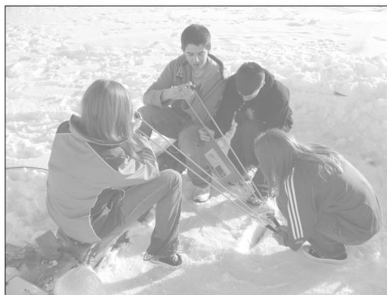
**The Air Resistance Lab** Joe DeLuca and Sheridan Monroe (with friends to help) conduct their experiment to determine how air resistance affects the distance that different balls will travel when launched at a constant force (using a water balloon launcher on the football field...in the snow!). Team member Kareem Shaban (not shown) is downfield noting the balls’ landing.
